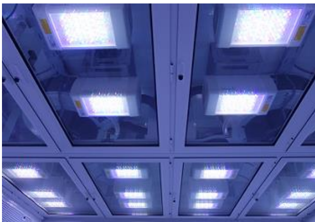
High performance LEDs with user adjustable spectral distribution
