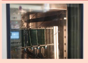
The observation window is composed of a multilayered glass with optimum levels of thermal insulation. The interior and exterior glasses have a heating system that is activated in cold cycles and damp heat to prevent condensation at the surface.
